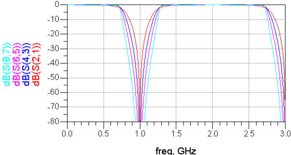
The plots above are for four different notch filters from n=2 to n=5, simulated with ideal transmission lines shown below. Each line is 90 degrees at the wanted frequency, and the results are in excellent agreement.
