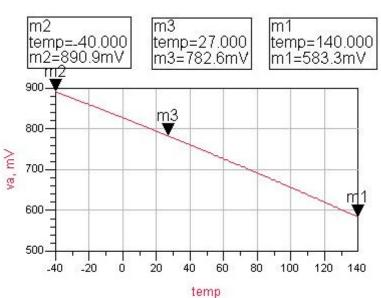
The plot shown here on the right is from ADS for the diode circuit shown at the top of the sheet.
