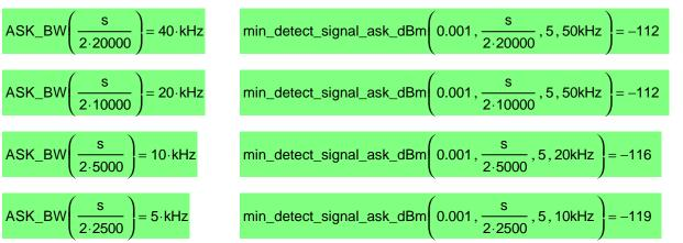
These figures show that the sensitivity and BW for different data rates. The 2 in the data rate for the bit period because the system is manchester encoded.
