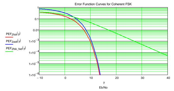
RED curve is with average white gaussian noise for 2FSK (frequency shift keying) BLUE curves with average white gaussian noise for ASK (amplitude keying or on/off keying) GREEN curve is with Raleigh fading for 2FSK
